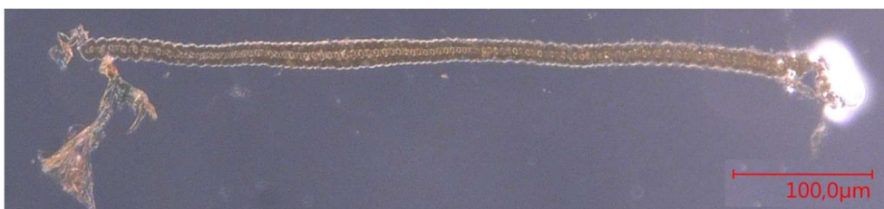
Figure 3.16: Amorphous, yellow, glass-like rod-material formed from [\text{Zn}_2\text{L}^{\text{crown}_3}_2] with NaCl in DMSO and benzene as anti-solvent.
