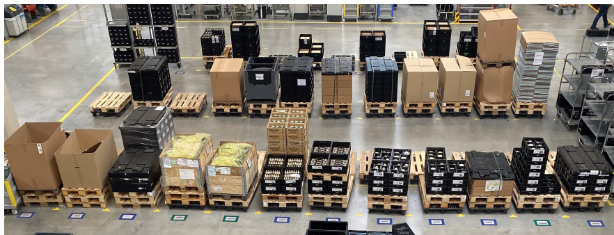
Fig. 2.6 Top view on a buffer storage for the material supply of a production system at a manufacturer of technical equipment.
