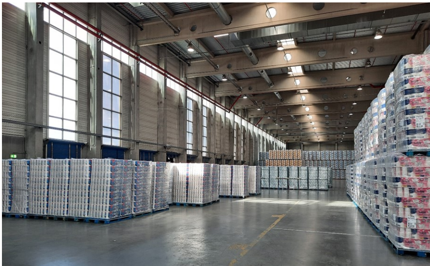
Fig. 2.4 Loading zone of a block stacking warehouse for finished goods at a hygienic paper manufacturer.
