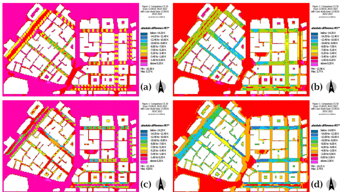
Figure 24. \Delta PET at Z = 1.5 m for the 20% and 50% tree scenarios compared to the 0% tree scenario for all aspect ratios and orientations at 12:00 (a,b) and at 15:00 (c,d).
