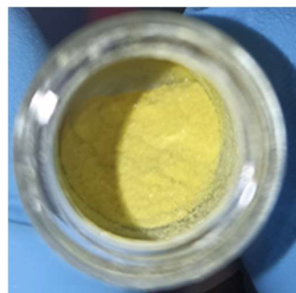
Figure 59: Yellow color of the synthesized Ni(cod) 2 25 indicates high purity. (Grey or beige color indicates the presence of metallic nickel, whereas green color indicates Ni(II) complexes).
