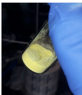
Figure 59: Yellow color of the synthesized Ni(cod) 2 25 indicates high purity. (Grey or beige color indicates the presence of metallic nickel, whereas green color indicates Ni(II) complexes).
