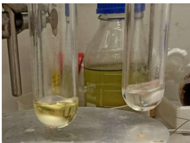
Figure 30: Catalyst preforming solutions partially deactivated (left) and non-deactivated (right).
