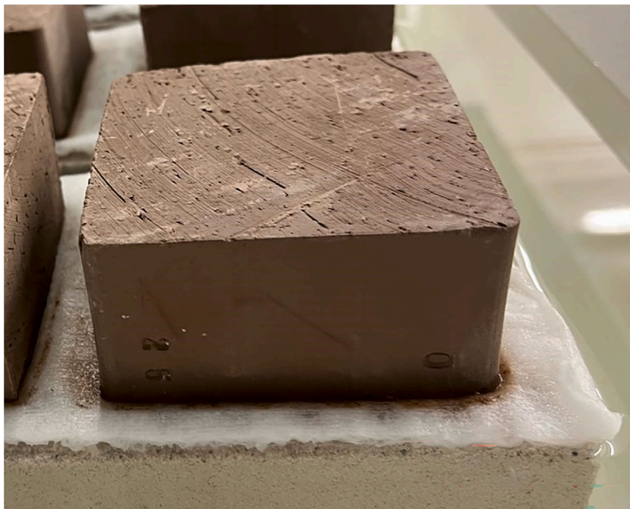
Fig. 6. Experimental setup for capillary water absorption testing.
