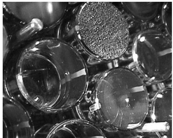
Fig. 36. Example of an undamaged PMT (left), a “frosty” PMT (top), and a “milky” PMT (bottom), observed in the drained SOB roughly one year after it was first filled with ultra-pure water.
