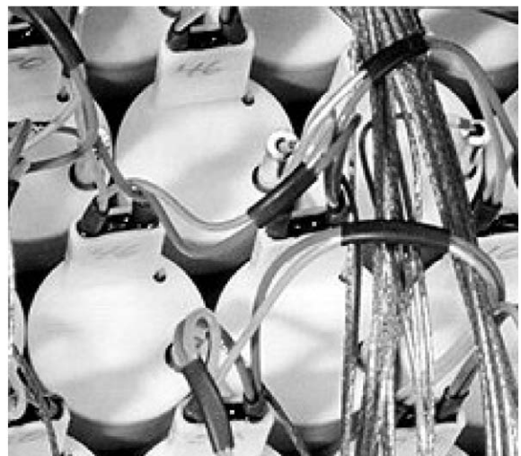
Fig. 37. Photograph of a group of DIRC PMT bases with signal and HV cables attached.
