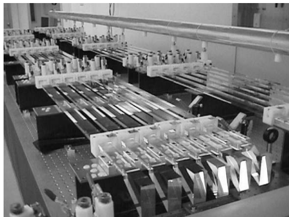
Fig. 29. A bar assembly station showing a set of six bars with wedges already attached.
