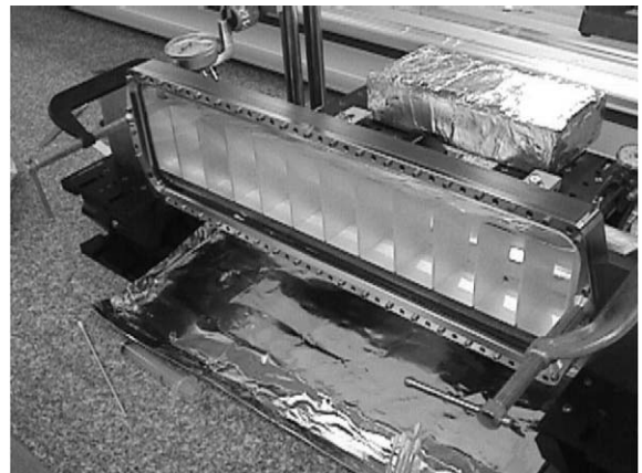
Fig. 28. End view of the window of a bar box showing the window-frame, fused-silica window and twelve wedges.
