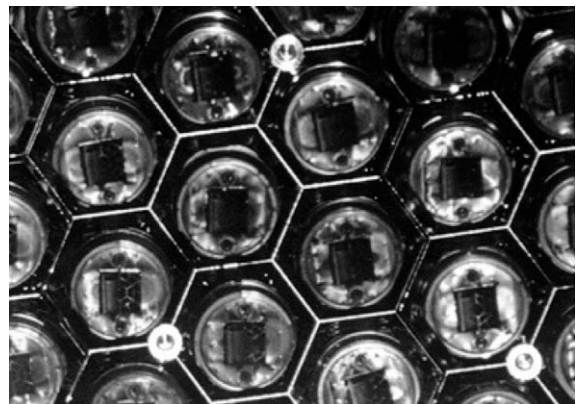
Fig. 39. PMTs and rhodium-plated light-catchers in the SOB.
