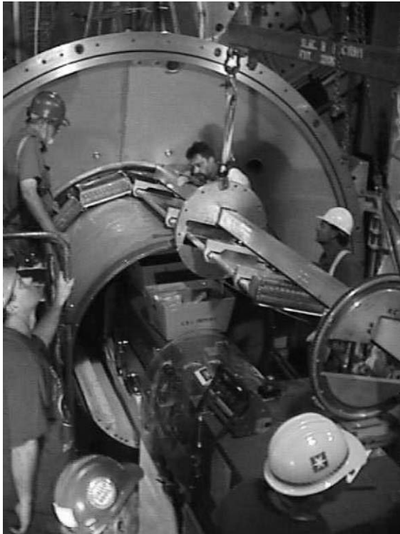
Fig. 30. Installation of a bar box into the BABAR detector. Not seen in the figures is the cantilevered support arm which supports the installation fixture above the accelerator components.
