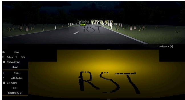
Figure 4.5.: Image GUI for pixel utilization control [Wal+23b].
