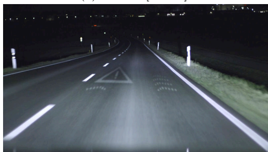
(c) Warning and guiding symbol projection [Aud22a].
