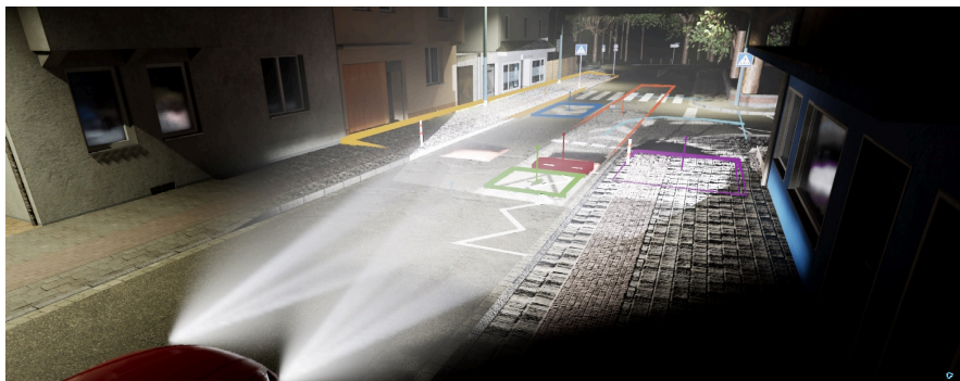
Figure 4.6.: Primitive GUI based on 3D primitives (colored boxes) for pixel utilization control, featuring volumetric fog simulation for beam propagation visualization [Wal+23b].
