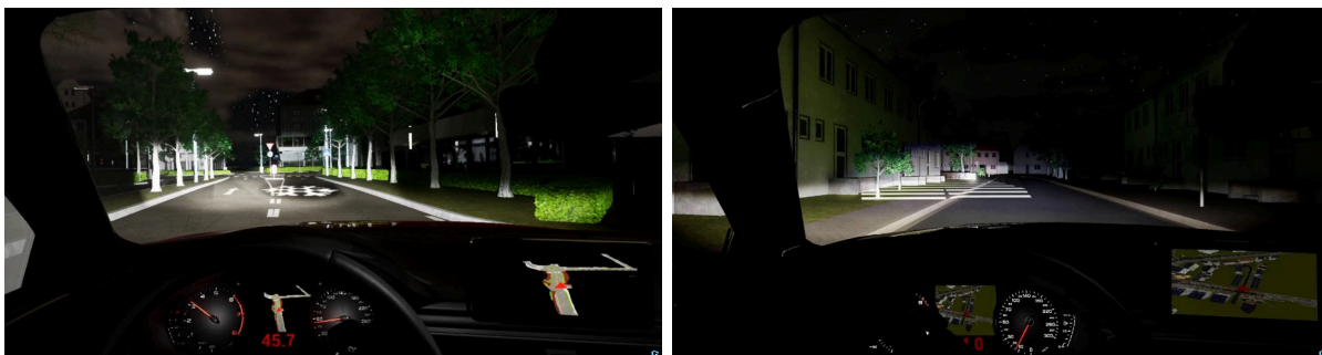
(a) Snowflake projection and bend lighting [Kau+24].
