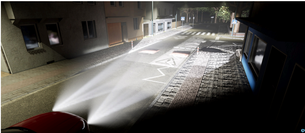
Figure 1.2.: SOL virtual environment impressions. Active lighting functions are selective lane and sidewalk illumination. In addition, the headlights project reversing arrows on the oncoming lane, a warning symbol in front of speed bumps and the planned route for turning right. A fog-like volume illumination simulation makes the beam spread visible [Wal+23b].
