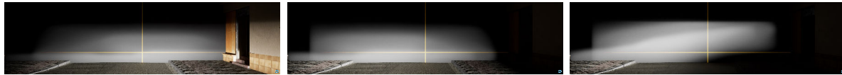
(a) Beam patterns of two modules (b) Digital bend lighting to the left side. (c) Combined digital bend, pitch and roll transformation.
