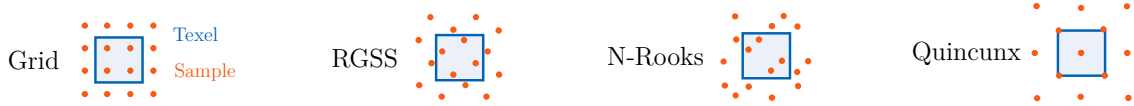
Figure 3.2.: SSAA grid patterns [Wik24; Ake+18]. The blue texel is sampled at the red locations.
