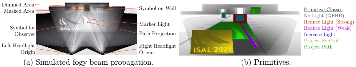
Figure 7.6.: SSC controls two matrix headlights with multiple primitives [WB22].
