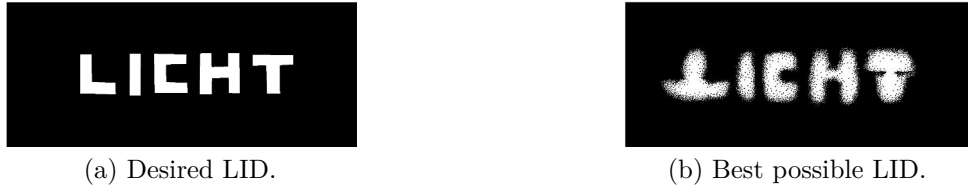
Figure 3.9.: Resulting possible LID from desired illumination [Hum+18]. As this Porsche patent [Hum+18] is from 2018, Fig. 3.9b seems to show the 3 \times 28 = 84 pixel HD84 headlight.
