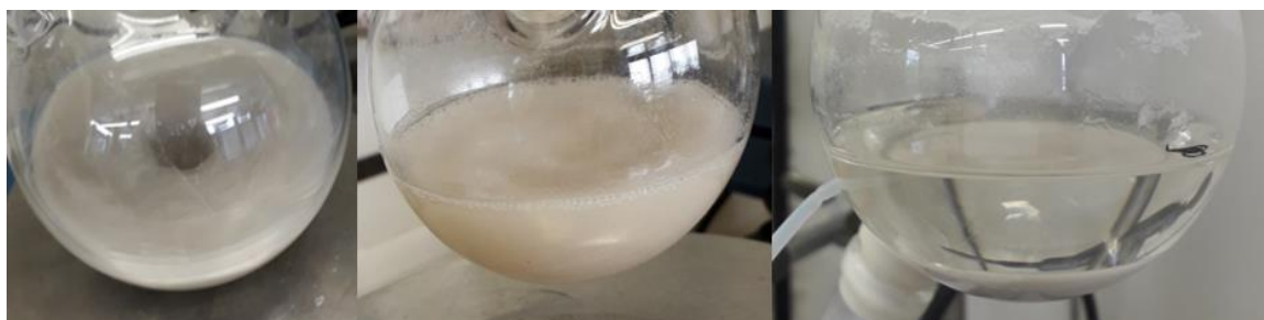
Figure 85: Sodium hydride suspension (left), addition of diethyl phosphonate (middle), after reaction (right) (from SCHMIDT 2020 109 ).
