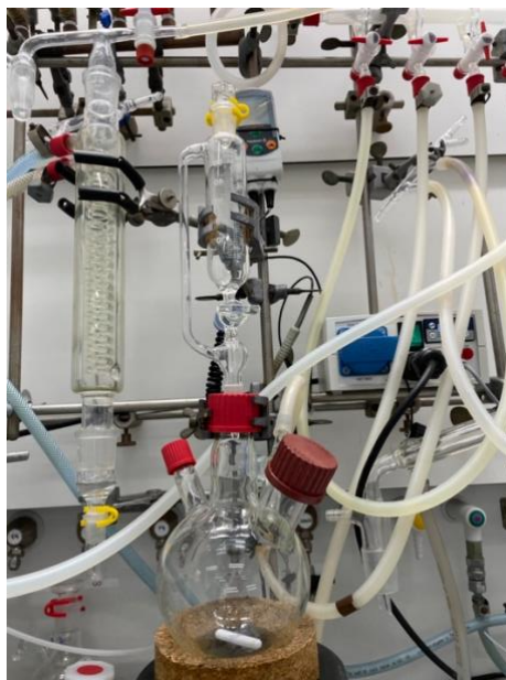
Figure 103: Apparatus for the reduction with DiBAL-H.
