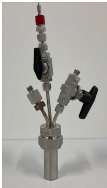
Figure 14: 25 mL autoclave for high-pressure catalytic experiments.
