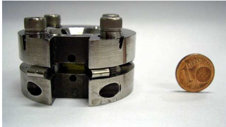
Figure 7.12: Mao–Bell diamond–anvil cell used during the high–pressure experiments. The picture shows a one–cent coin for size comparison.
