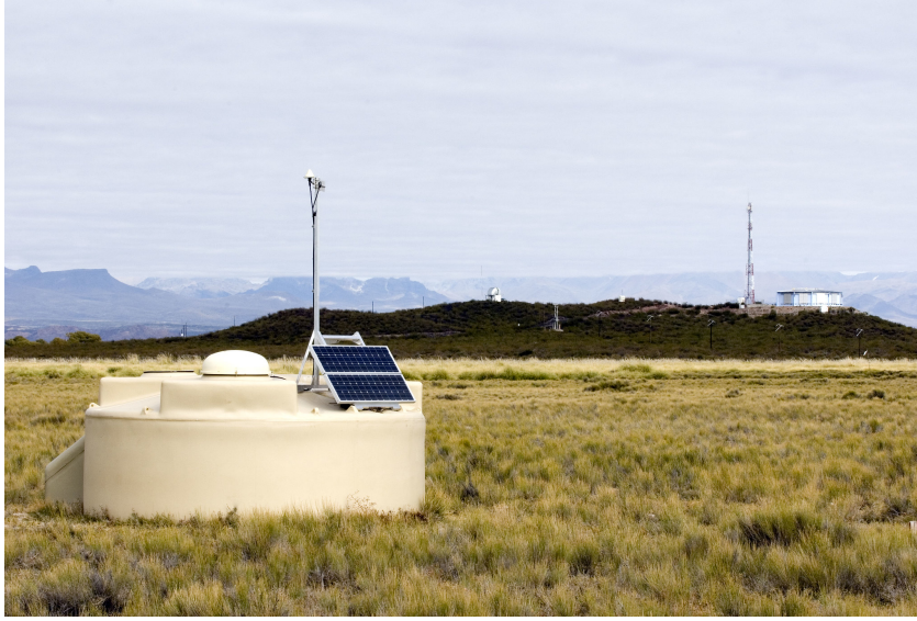
Figure 3.3: Photo of a Cherenkov detector used in the Pierre Auger Observatory. Picture is taken from Ref. [25].
