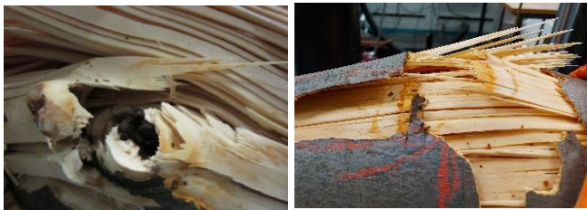
Figure 3 Damage patterns in the bending test on imperfect test specimens with branch hole and incipient callus formation (left) and fiber crushing (right). Source: Ingo Muench/TU-Dortmund
