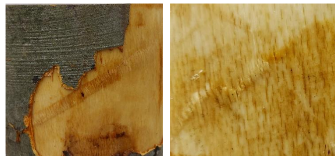
Figure 5 Damage pattern in the pure compression test (left) and in the compression zone of the bending test (right). Source: Ingo Muench/TU-Dortmund
