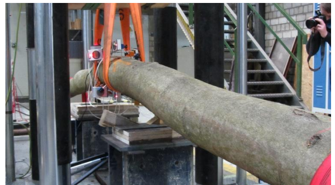
Figure 2 Ultimate load test on a whole stem under bending. Source: Ingo Muench/TU-Dortmund
