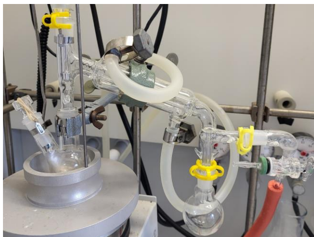
Figure S 8: Reaction set-up for the catalyst recycling experiment.
