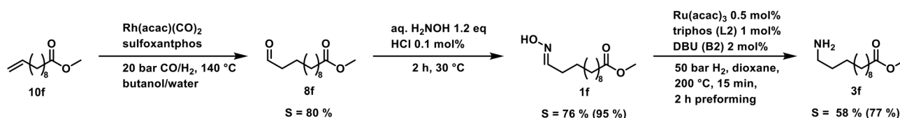
Scheme 5 Reaction sequence starting with a reaction solution sample of a continuously operated miniplant. Selectivity combined for the alkene and each reaction in parentheses.
