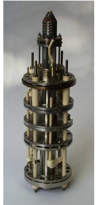
Figure 3.4: Picture of ion lens system.
