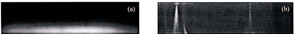
Figure 4.6: Typical 10 ns exposure time photographs of a 4 mm gas gap during: (a) an atmospheric pressure glow discharge (APGD) ( V_{max}=11 kV) (b) a filamentary discharge ( V_{max} = 14 kV) [Ghe00]
