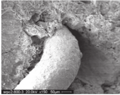
(a) Steel fibre-reinforced reactive powder concrete (RPC). Reprinted from [179], copyright (2013), with permission from Elsevier.
