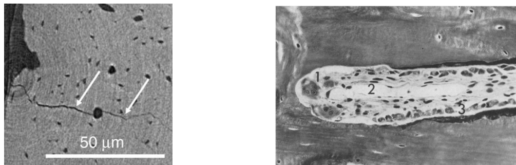
(a) CT image of microcracks in the mid-diaphyseal, cortical cross section of a mouse femur. The cracks occurred in consequence of compressive loading in an experimental setup in vitro. Reprinted from [166], copyright (2009), with permission from Elsevier.
