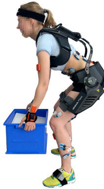
Figure 1. Task 1: lifting and lowering a box with the exoskeleton PaexoBack.
