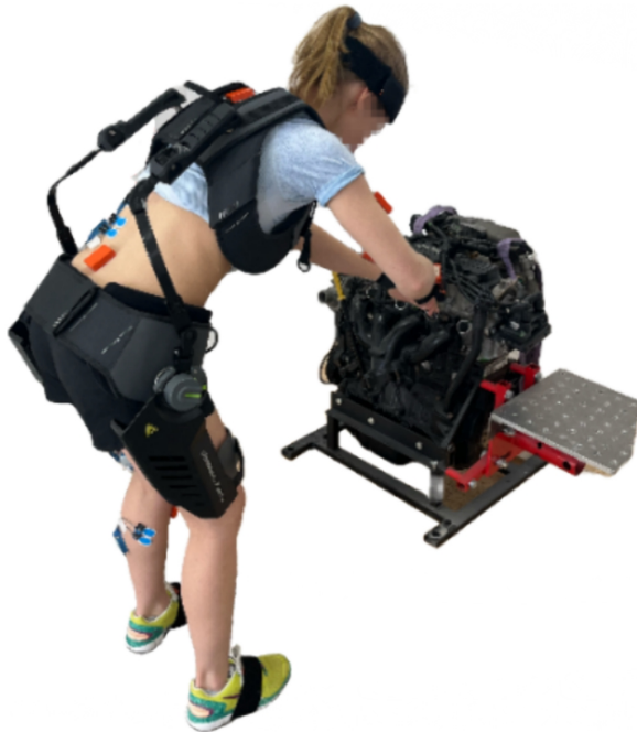
Fig. 4. Task 4: Static bending task with the exoskeleton PaexoBack.
