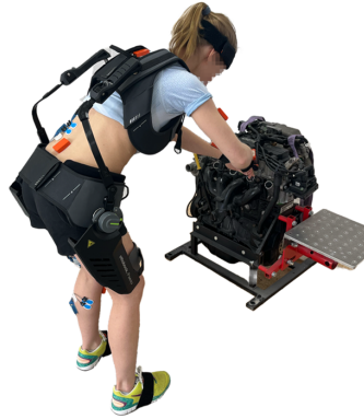
Figure 3. Task 4: Static bending task with the exoskeleton PaexoBack.
