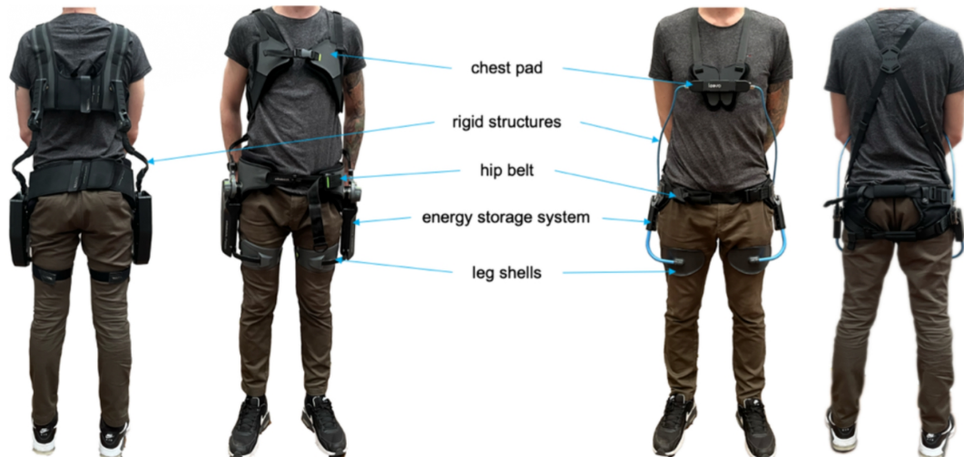
Fig. 1. In this study used BSEs with their components, PaexoBack (left) and Laevo (right).
