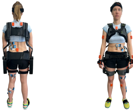
Figure 4. Sensor placement of sEMG and Xsens sensors.
