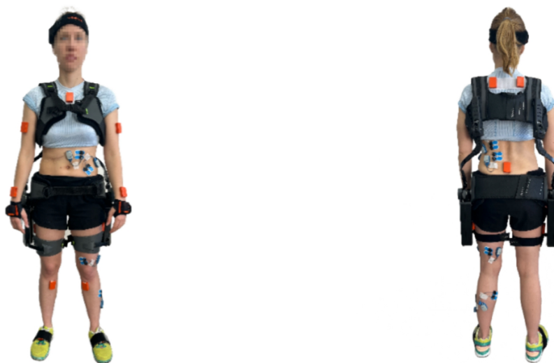
Fig. 5. Sensor placement of sEMG and Xsens sensors.
