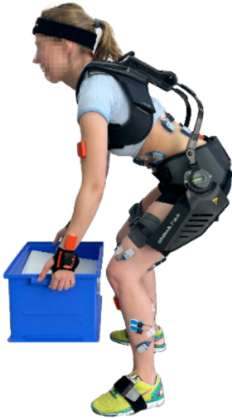
Fig. 2. Task 1: Lifting and lowering a box with the exoskeleton PaexoBack.
