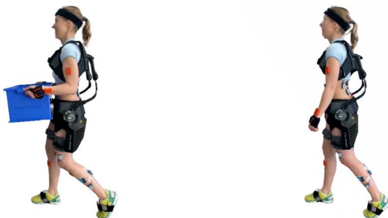
Fig. 3. Task 2 and 3: Carrying a box (left) and walking without load (right) with the exoskeleton PaexoBack.
