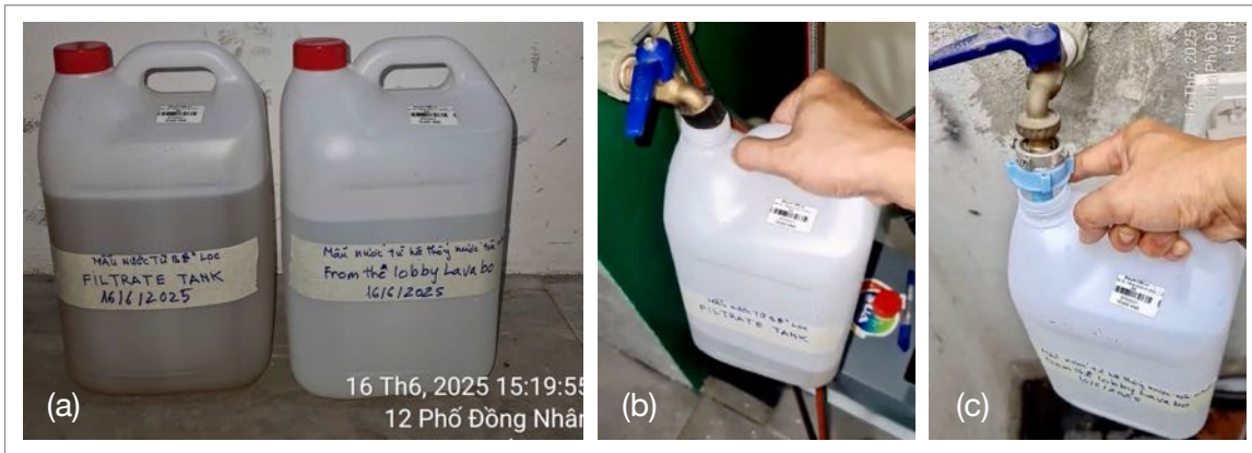
Figure 5.12: Filtrate Examples for Water Quality Certificates, 16.06.2025. (a) both Samples in 2 Liter Canisters, (b) Sample of Filtrate, (c) Sample of Tap Water
