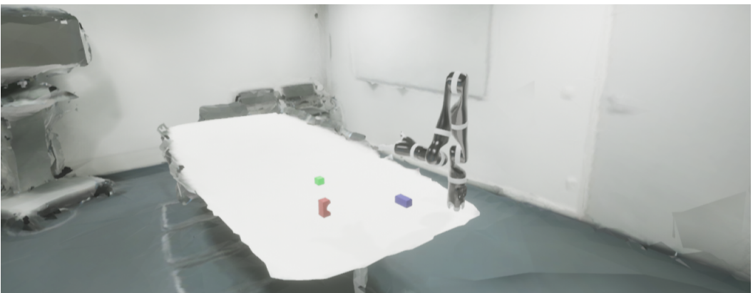
Fig. 8. Example scenario provided in AdaptiX including a table, a virtual Kinova Jaco 2 robotic arm and colored blocks on the tabletop.
