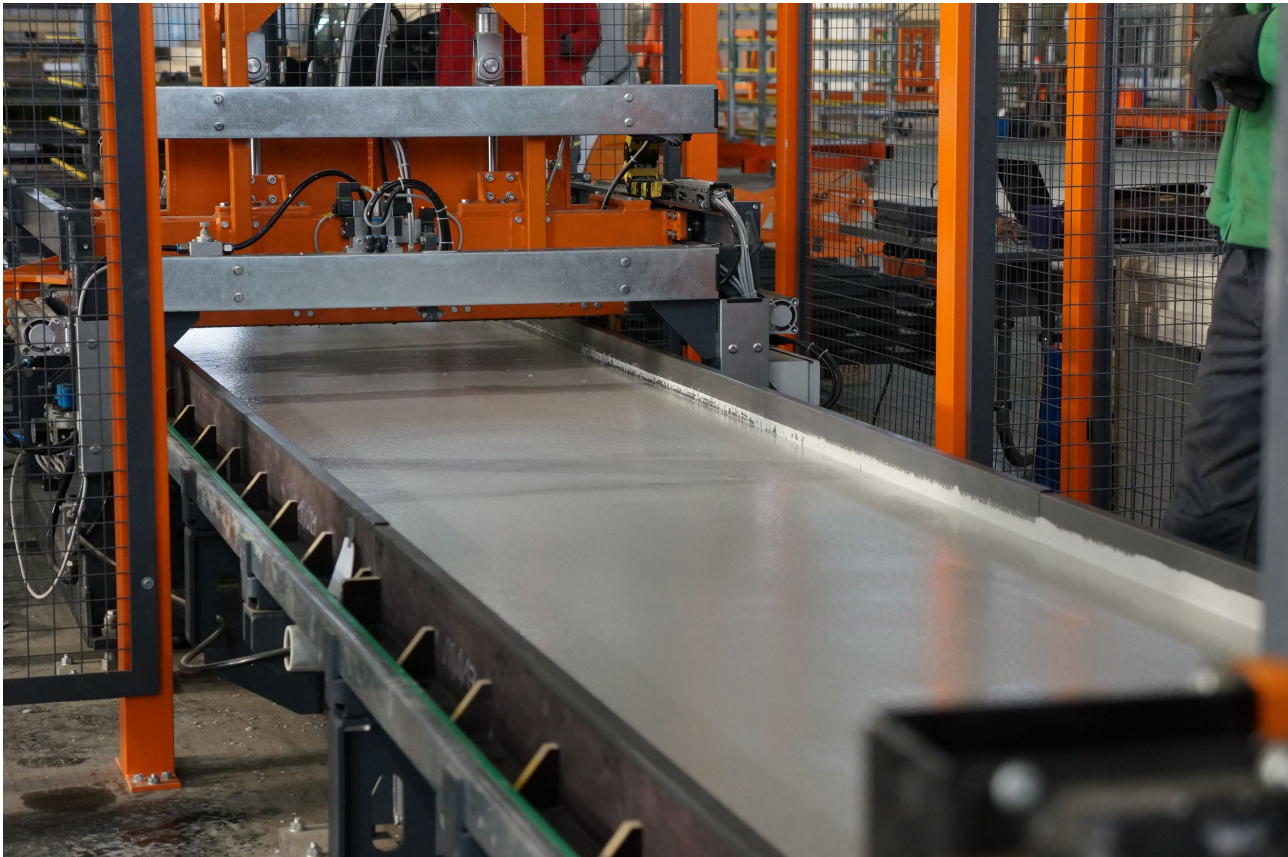
Abb. 16: Co-Extrusions-Technologie, Aeroleichtbeton © G.tecz Engineering GmbH
