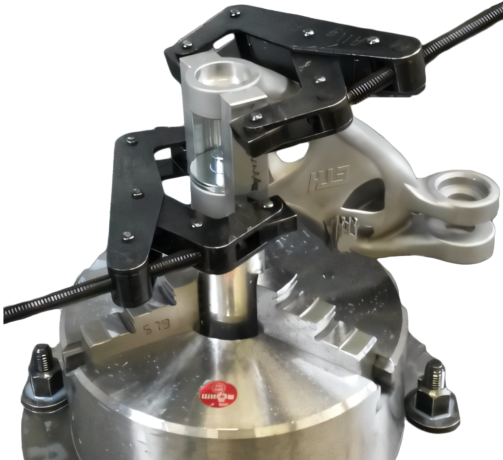
Figure 2.2: Example of complex clamping solution [47]
