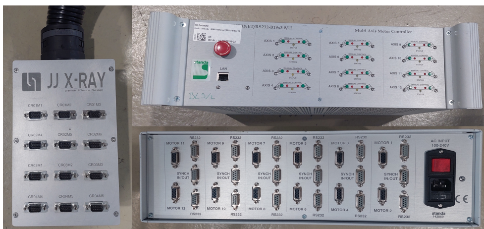
Figure A.1: left) Motor-box of the von Hámos spectrometer for moving the individual motors for the crystals. right) Standa controller for controlling the motor movement of the crystal motors. top front view bottom backside view.
