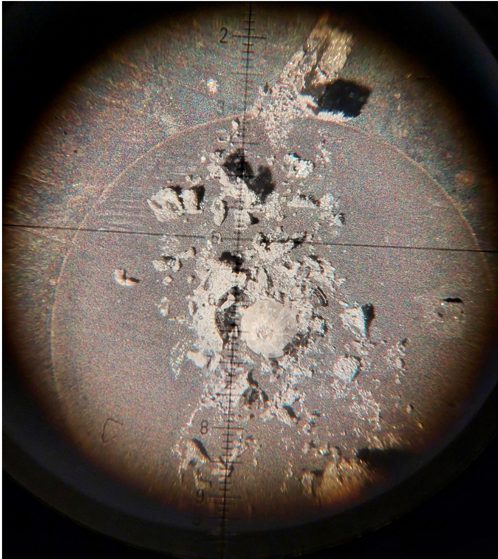
Figure A.12: Photo of nearly only diamond dust. The pavilion planes and culet are still recognizable, but the outer parts are scattered across the seat.
