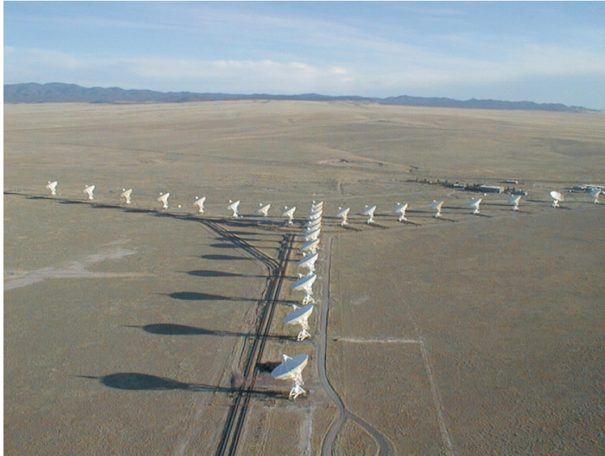
Figure 2.2: Aerial overview of the VLA. The antennas are mounted on rails and arranged in a Y formation. [82]
