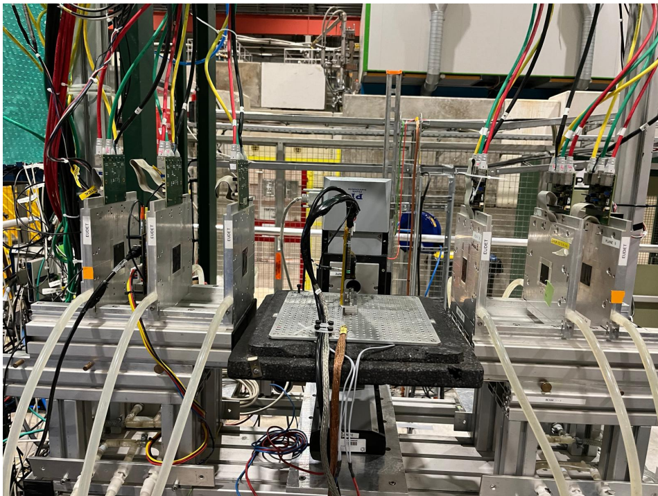
Figure B.1: Photo of the beam test setup including the tracking planes and the SINTEF 3D module as DUT.
