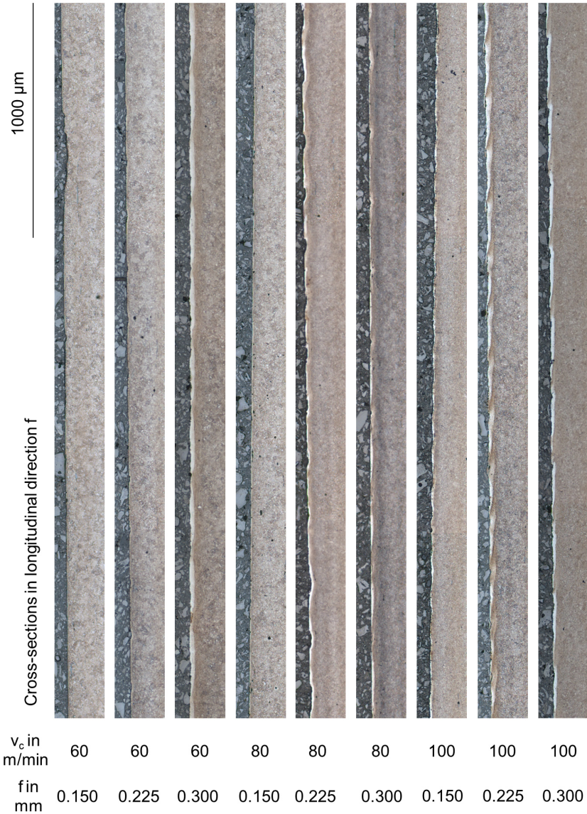
Figure 5.19 Large-scale micrographs of cross-sections in the longitudinal direction of specimens drilled at varying cutting speeds ( v_c = 60\text{-}100 m/min) and feeds ( f = 0.150\text{-}0.300 mm) (batch A)
