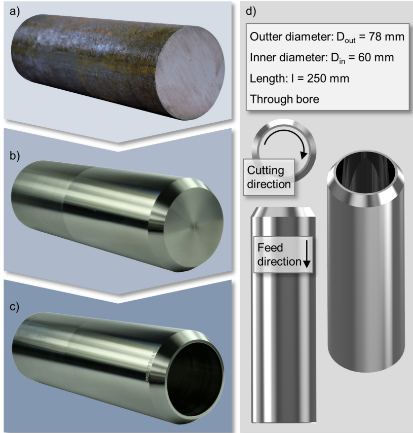
Figure 3.5 Preparation of specimens: a) Rolled round bars; b) turned round bars; c) BTA deep drilled round bars; d) specimen geometry and direction of feed and cutting
