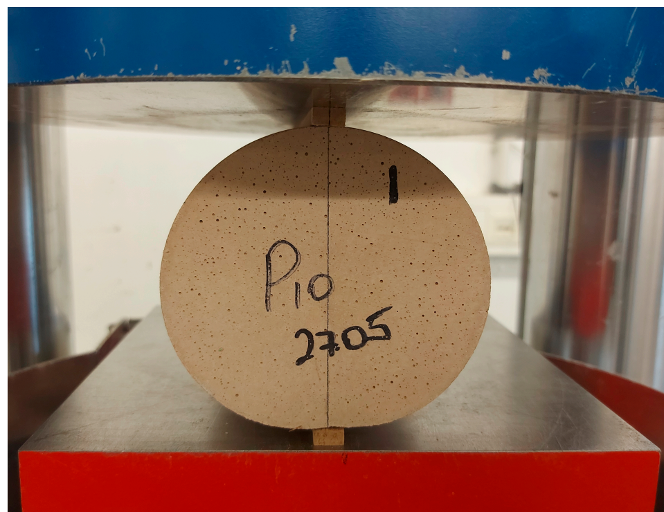
Figure 5. Splitting tensile strength test (mixture No. 10).
