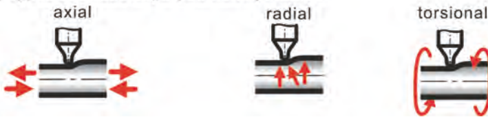
(b) Types of stress superposition \sigma_0 studied
