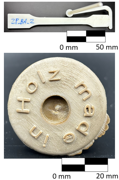
FIGURE 3 | Molded parts. Top: Tensile test specimen made of ABS in bamboo mold (T_BA_ABS_2), Bottom: Logo specimen made of PEEK in birch mold (L_BI_PEEK_1).
