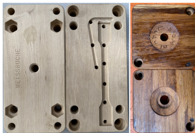
FIGURE 1 | Inserts for different specimen types. Left: Insert for tensile test specimen made from Hornbeam. Right: Insert for Logo-Specimen made from compressed bamboo.
