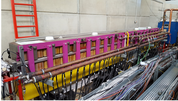
Figure 3.4: Electromagnetic undulator U250 offers two different modes of operation: it can either be used as one long modulator or it is powered in a segmented way such that three regions are powered as modulator, chicane and radiator (see text for details).
