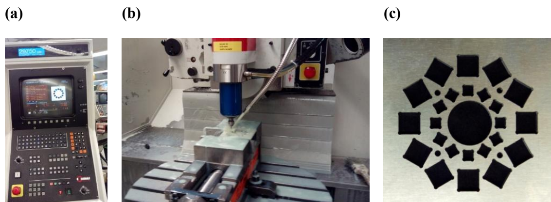
Figure 4.2: (a and b) Computerized grinding machine located in ISAS demonstrating the process of preparing one aluminum plate with the Halbach array pattern as depicted in (c).
