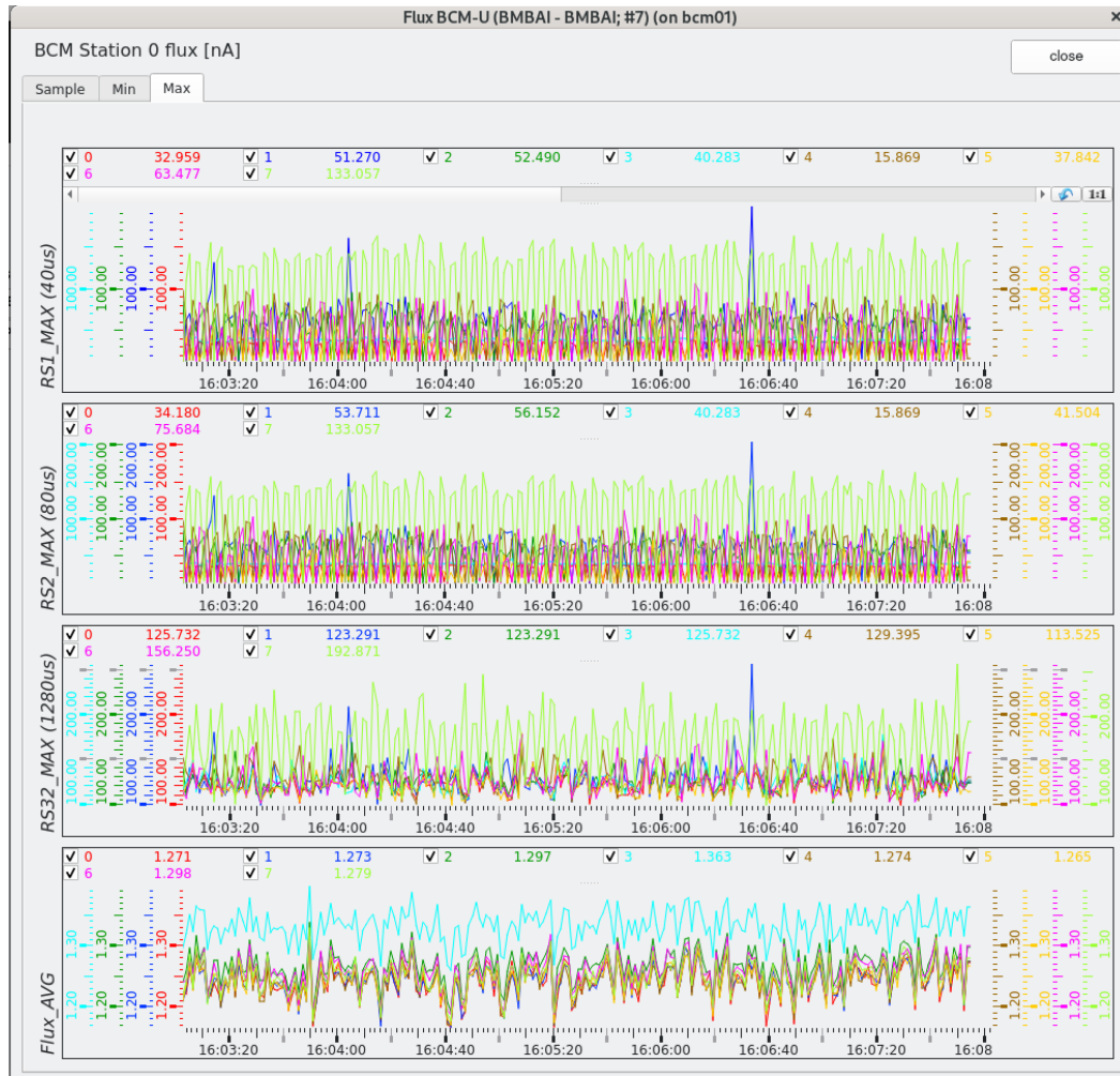
Figure 4: The detailed currents of the BCM-U station showing the values for RS1, RS2, RS32 and the average flux.
