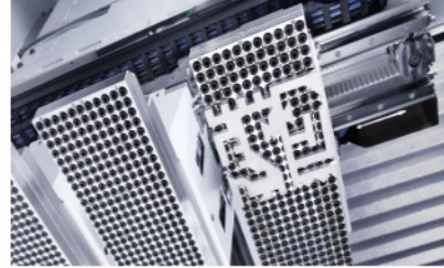
Fig. 2.6: Part Handling with the SortMaster Speed. Source: TRUMPF.
