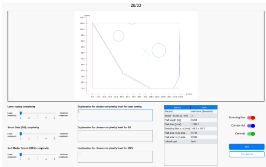
Fig. 4.7: Interface of the Labeling Tool. Own visualization.
