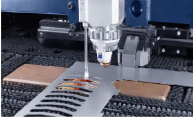
Fig. 2.5: Part Handling with the SmartGate. Source: TRUMPF.
