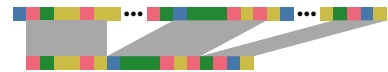
Figure 1.13: A read (bottom) is mapped to a reference sequence (top). In this example, the read consists of 3 separate parts, each of which maps to a different region in the reference, and is hence labelled as a split read .
