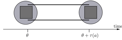
Figure 1.2: Arc with transit time \tau(a) in a discrete flow over time model. Flow units leaving a node via arc a at time \theta \in \{0, 1, \dots, T - 1 - \tau(a)\} totally have left arc a at time \theta + \tau(a) .
