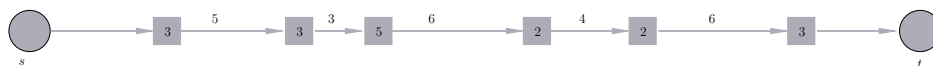
Figure 5.1: Path representing a data transmission from the source to the sink via several processors. The numbers in nodes represent the capacity of the processor and number on arcs represent the transit time data needs to travel from one processor to the next one.
