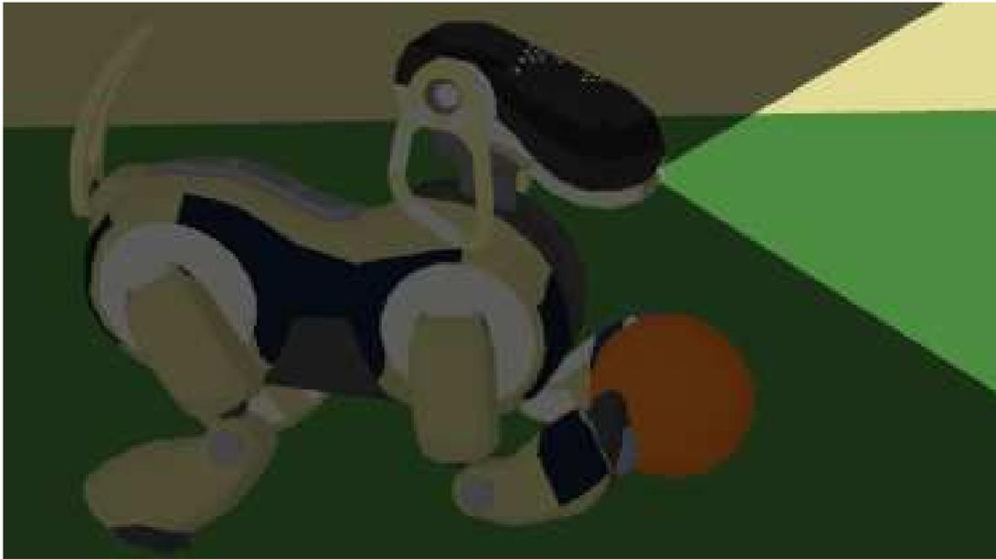
Figure 3.6: An Aibo which turns around a ball and cannot see it. To illustrate this the opening angle of the camera is lit.
