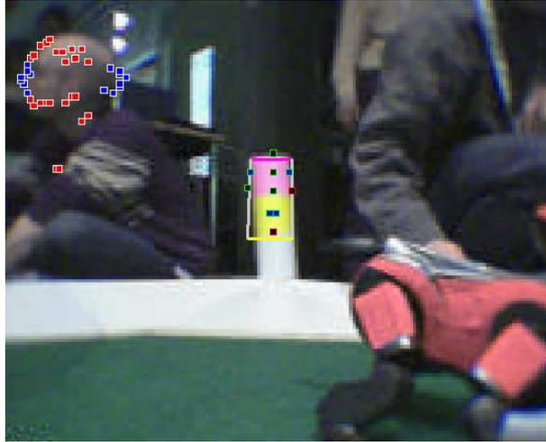
Figure 4.9: A beacon detected by the Box specialist. The points represent edges
