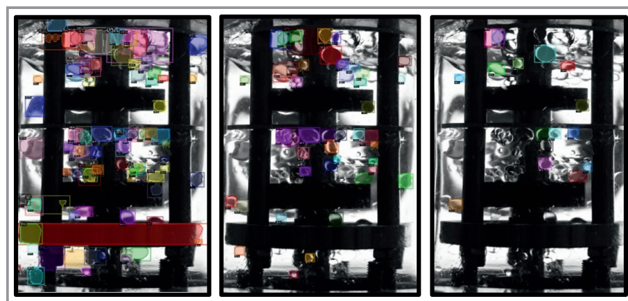
Figure 3. Results of Mask R-CNNs droplet detection for different confidence thresholds, left side IOU = 0.1, central image IOU = 0.25, right side IOU = 0.4 set as threshold.
