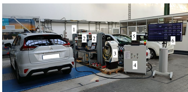
Fig. 2 Laboratory setup, 1: Wirelane charger, 2: KoCoS power quality analyser, 3: EVTEC charger, 4: EV monitoring system, 5: User interface, 6: Monitoring dashboard.
