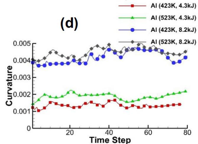
*(a) & (c) SNI plots, (b) & (d) Curvature plots for runs with Mg-alloy & Al-alloy respectively for fully Clamped end condition.*
