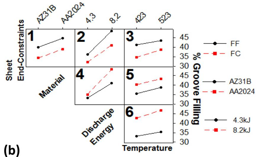
(a) Main effect plots, (b) Interaction plots, of all the factors taking maximum filled groove height/Total groove height as a response.
