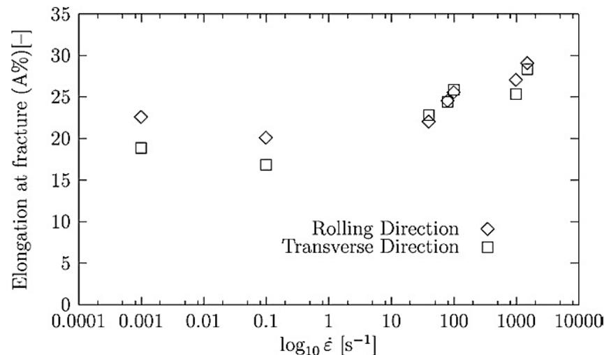
Elongation at fracture at room temperature for different strain rates
