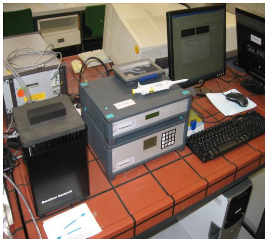
Figure 2.6: The picture of TF Instruments Ultrasonic Resonator in our laboratory.
