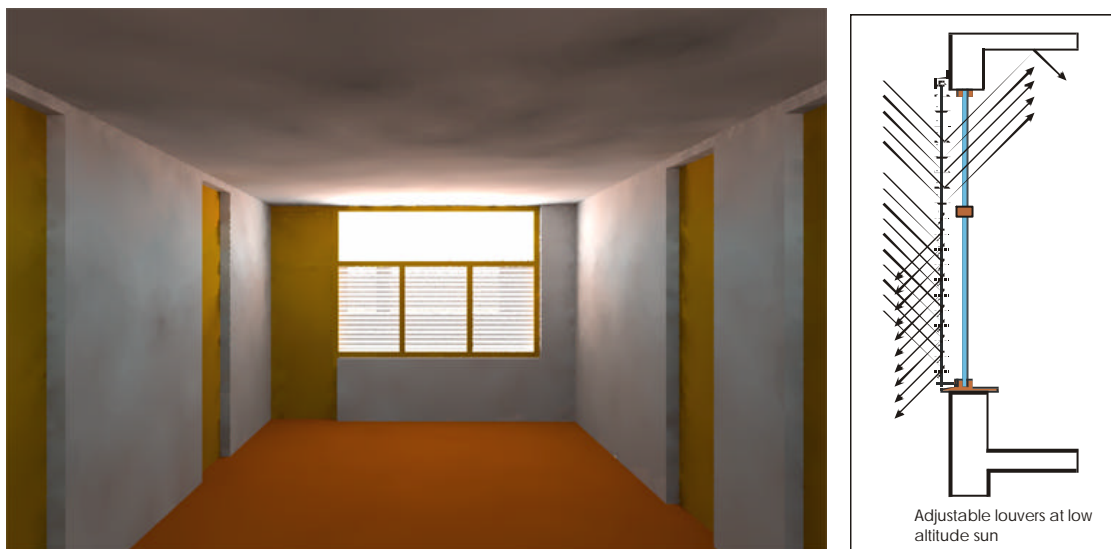
Figure 4.22: Visualisation diagram showing illumination of a room facing east without a roof projection but with an adjustable louver screening device on the window which redirects light to the ceiling
