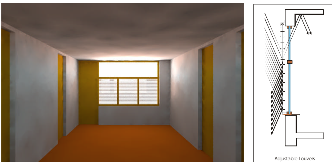
Figure 4.19: Visualisation diagram showing illumination of a room facing north without roof projection but with a modified louver screening device on the window which re-directs light to the ceiling
