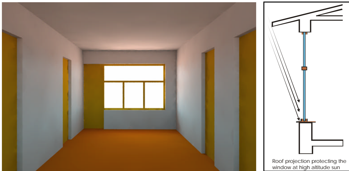
Figure 4.16: Visualisation diagram showing the effect of a roof projection on illumination in a room facing north under clear sky conditions without considering extra solar screening device on the window
