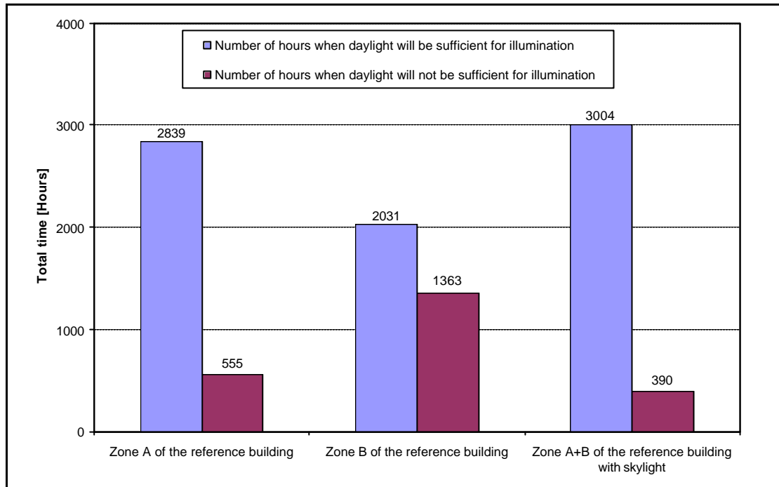
Figure 8.4: The time when light will be sufficient for illumination in a building with and without a skylight.
