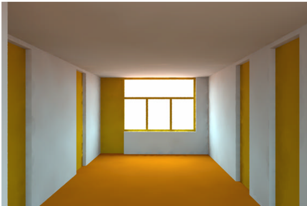
Figure 4.14: Visualisation diagram showing illumination of a room facing north under overcast sky conditions without considering solar screening device on the window
