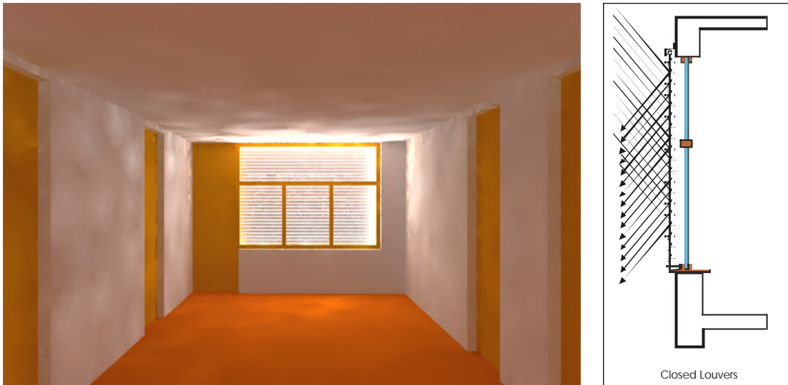
Figure 4.18: Visualisation diagram showing illumination of a room facing north under clear sky and a solar screening device (louvers) with closed lamellas
