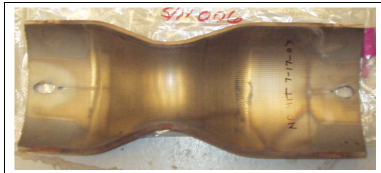
Figure 8: Small rocket nozzle panel.
