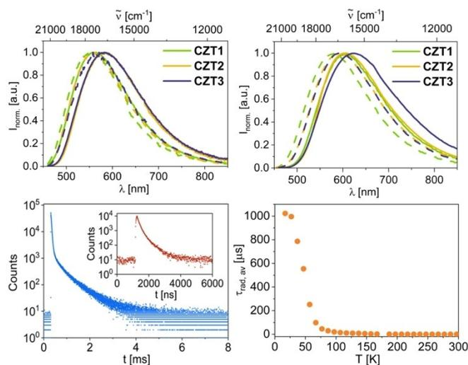
**Figure 2.** Top left: Photoluminescence of **CZT1–3** in the solid state at room temperature (dashed lines) and at 77 K (solid lines). Top right: Photoluminescence of **CZT1–3** in 1 wt% PS (solid lines) and PMMA (dashed lines). Bottom left: Photoluminescence decay of **CZT2** at 77 K and 297 K (inset) in the solid state. Bottom right: temperature-dependence of the averaged radiative lifetimes  $\tau_{\text{av,rad}}$  of **CZT2**.
