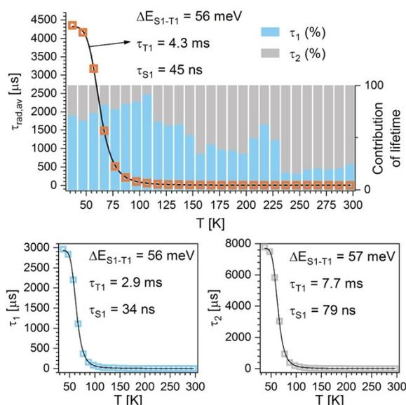
**Figure 3.** Top: Temperature-dependence of the averaged radiative lifetime  $\tau_{rad,av}$  of **CZT3b** and relative contributions of  $\tau_1$  and  $\tau_2$ . Bottom: Temperature-dependence of  $\tau_1$  and  $\tau_2$ . The black lines represent the fit of the experimental data according to eq 1, and the obtained fitting parameters of the TADF are given in the graphs.
