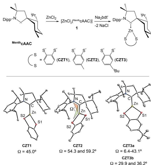
**Scheme 2.** Top: Synthesis of **1** and CZT1–3. Bottom: Molecular structures of CZT1–3 and their dihedral angles  $\Omega$ . Hydrogen atoms are omitted for clarity.
