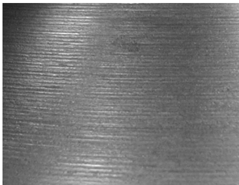
Fig. 7a. Rills caused by roller tool indentations
