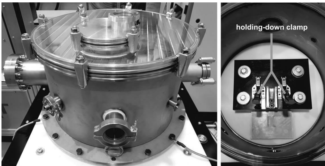
Figure 2: vacuum chamber designed for MPW (left: vacuum chamber with cover, right: coil and holding-down clamp)
