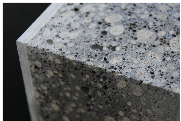
Fig. 8 Material sample of the ‘lightweight aero concrete’ mixture. The hybrid component shows the outer UHPC layer and the lightweight porous core © G.tecz Engineering GmbH
