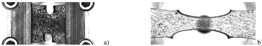
Fig. 1: Photos of the tensile test with inhomogeneous deformation states of a notched specimen a) at the beginning of the experiment at t = 2.55 s and b) before the sample starts to tear at t = 1139.8 s; cf. [6].
