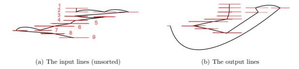
Figure 4.15: An illustration of the sorting algorithm using Line Pairs
