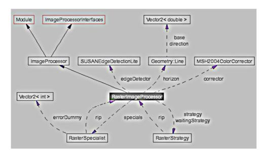
Figure 4.6: Collaboration diagramm for class RasterImageProcessor.
