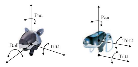
Figure 3.11: 3 headjoint values pan tilt and roll. The roll joint of the ERS-210 had changed to tilt2 in the ERS-7
