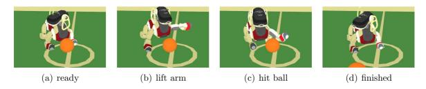
Figure 3.14: The *MSH7SlapLeft* was created to quickly move the ball from the border by hitting it from above with the left arm.
