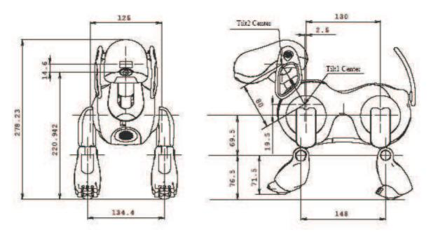
Figure 3.2: Technical drawing of the front and side of the ERS-7 robot. All measurements given in mm.
