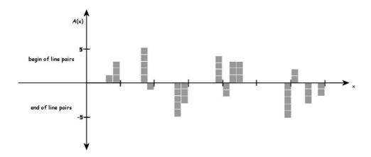
Figure 4.25: Array A[] after Line Pairs were collected. The x-axis displays the scan line, the y-axis shows the amount of startings (positive) or endings (negative) of an amount of Line Pairs in the image. Gray squares stand for an increment/decrement, which has taken place.
