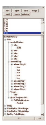
Figure 5.2: A screen shot of the tactic-entry editing window. The entries currently loaded define the behavior for the open challenge (see 7.3.2 on page 83).
