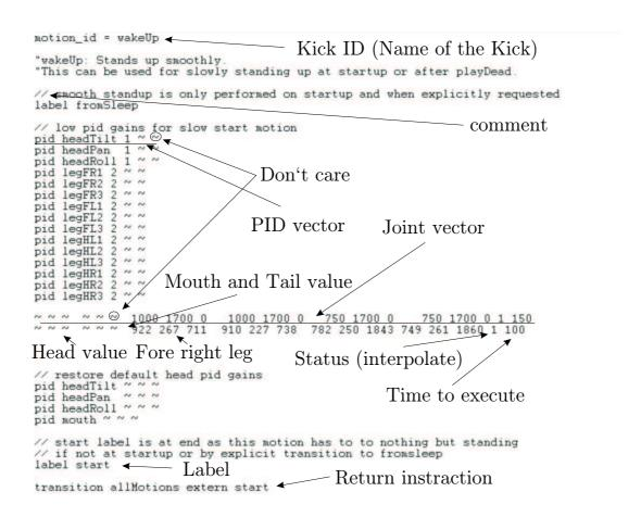
Figure 3.7: "wakeUp" mof as example for a motion file
