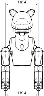
Figure 3.1: Technical drawing of the front and side of the ERS-210 robot. All measurements are given in mm.
