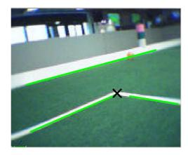
Figure 4.11: The goal area corner has been detected
