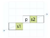
Figure 4.4: Scan line filter - Note, that p is the considered pixel. The green pixels represent the neighbourhood used to calculate the *edginess*. The other highlighted pixels belong to the scan line.
