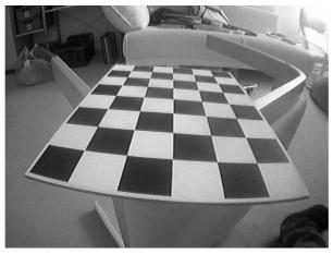
(a) Calibration object - note that the checkerboard's edge appears bent though it is perfectly straight in reality
