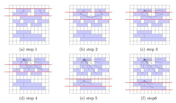
Figure 4.8: Illustration of the region merging algorithm.
