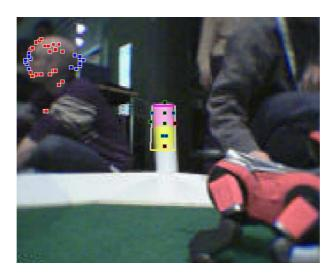
Figure 4.9: A beacon detected by the Box specialist. The points representes edges
