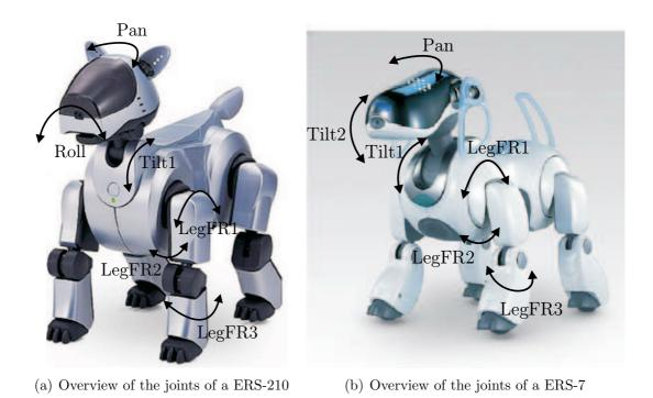
Figure 3.8: overview of the joints of ERS-210 and ERS-7. The roll joint of the ERS-210 has changed to a tilt2 joint of the ERS-7
