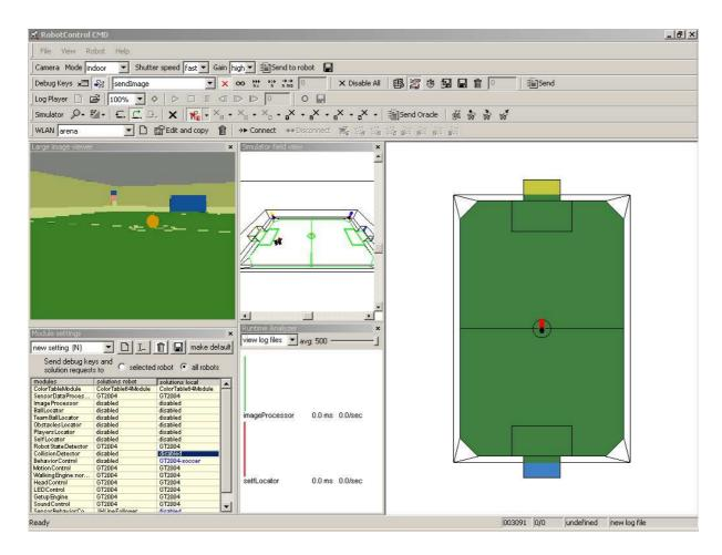
Figure 2.3: Screenshot of RobotControl, the application which is used for debugging
