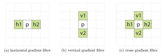
Figure 4.3: Basic gradient filters - Note, that p is the considered pixel. The green pixels represent the neighbourhood used to calculate the *edginess*.
