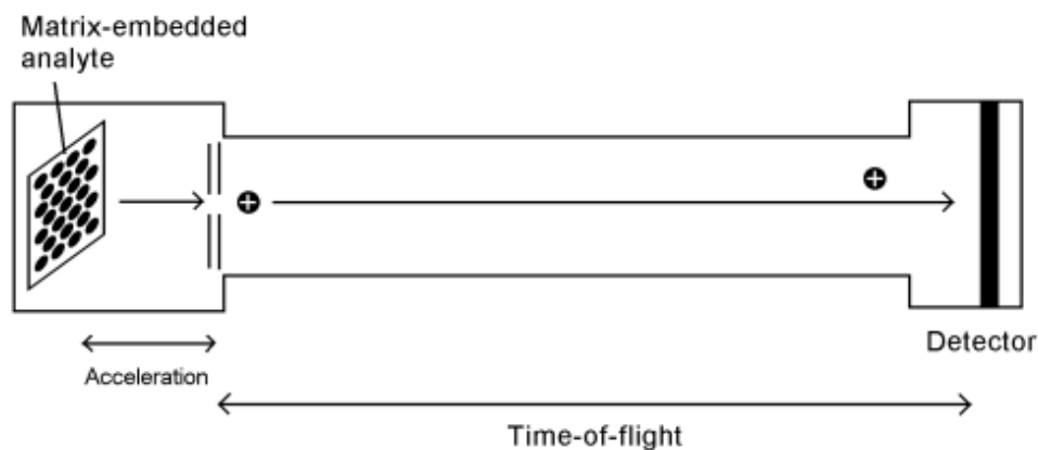
Figure 2.13: Workflow of Matrix-Assisted Laser Desorption/Ionization Time-Of-Flight mass spectrometry (graphic modified from Pusch et al., 2003).
