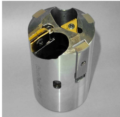
Figure 5.7: BTA deep-hole drilling tool as used for the experimental investigation
