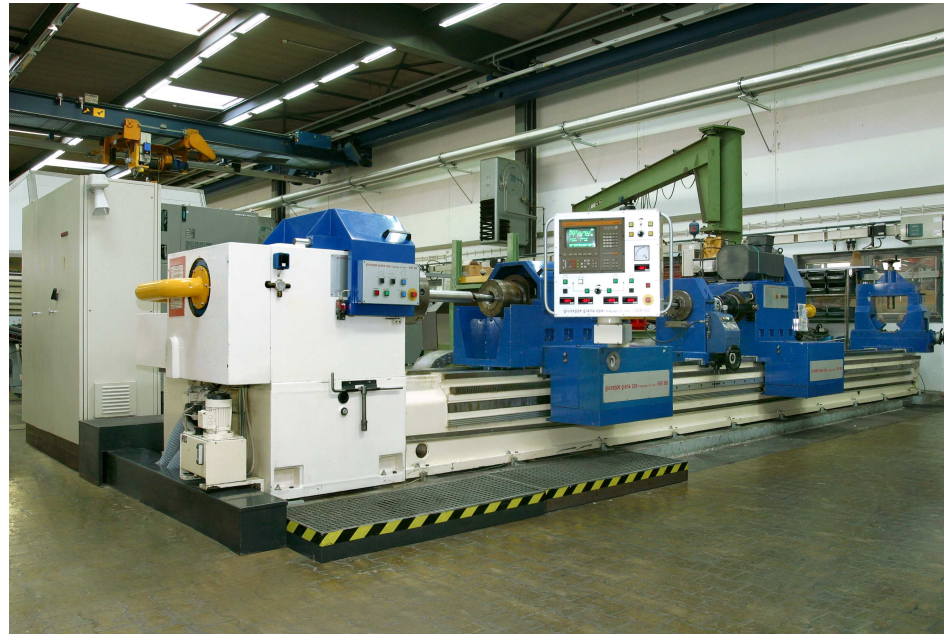
Figure 5.6: Deep-hole drilling machine Giana GGB 560
