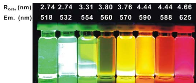
Figure 2.1.5 Color photograph demonstrating the size-tunable fluorescence properties and wide spectral range of the eight QD dispersions (CdSe or CdSe/ZnS) plotted versus CdSe core size and emission maximum. The samples were excited using a 365 nm UV light.
