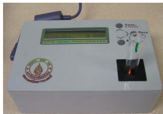
Figure 3: Portable MT photometer used for measurement of xylose and ethanol contents.
